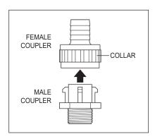
Wedgit Connectors are sold in four paired configurations. Each pair consists of a female coupler and a male coupler. The four pins located on the male coupler engage with the female coupler's internal wedge to lock/unlock the fitting. The inlet and outlet pairs are specially designed for error-free tank connections.
